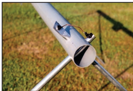
Figure 4 — One method of attaching a feed line. Flattened tubing end is drilled for a coax bulkhead connector. Exposed connections are covered with silicone sealant to prevent exposure to water and corrosion.
